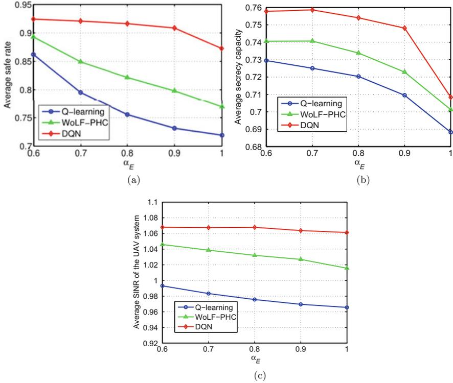
**Fig. 7** Average performance of the learning based power allocation strategy against smart attacks with  $P_T = P_J = 0.4$ ,  $L = 5$ ,  $\sigma = 1$ ,  $C_m = 1.5$ , and  $\alpha_A = 1$ . (a) Average safe rate. (b) Average secrecy capacity. (c) Average SINR of the UAV system
