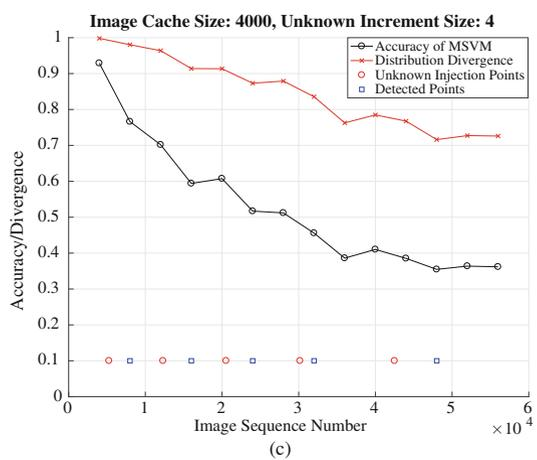
**Fig. 6** Unknown sample triage with varied image cache size  $s$  and a fixed unknown camera model increment size  $u$ . **(a)**  $s = 2000, u = 3$ . **(b)**  $s = 3000, u = 3$ . **(c)**  $s = 4000, u = 3$
