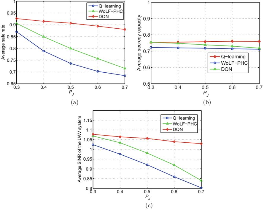
**Fig. 8** Average performance of the learning based power allocation strategy against smart attacks with  $P_T = 0.4$ ,  $L = 5$ ,  $\sigma = 1$ ,  $C_m = -0.5$ ,  $\alpha_E = 0.8$ , and  $\alpha_A = 1$ . (a) Average safe rate. (b) Average secrecy capacity. (c) Average SINR of the UAV system
