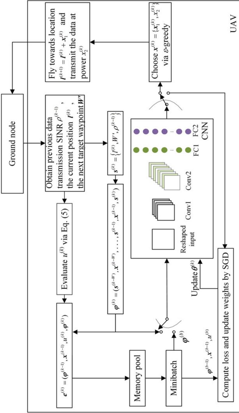
Fig. 1 RLTPC scheme for the UAV against smart jamming attack
