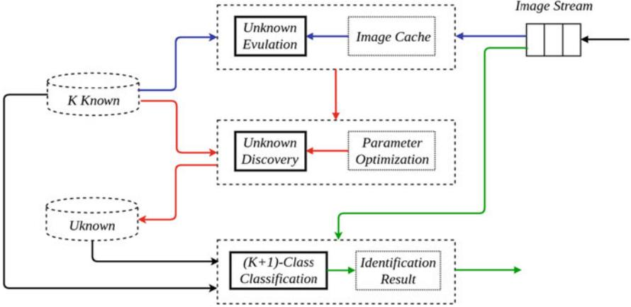
**Fig. 1** The system model of OSIU (the blue line, red line, and green line indicate the data flow of unknown sample triage, unknown image discovery, and  $(K + 1)$ -class classification, respectively)
