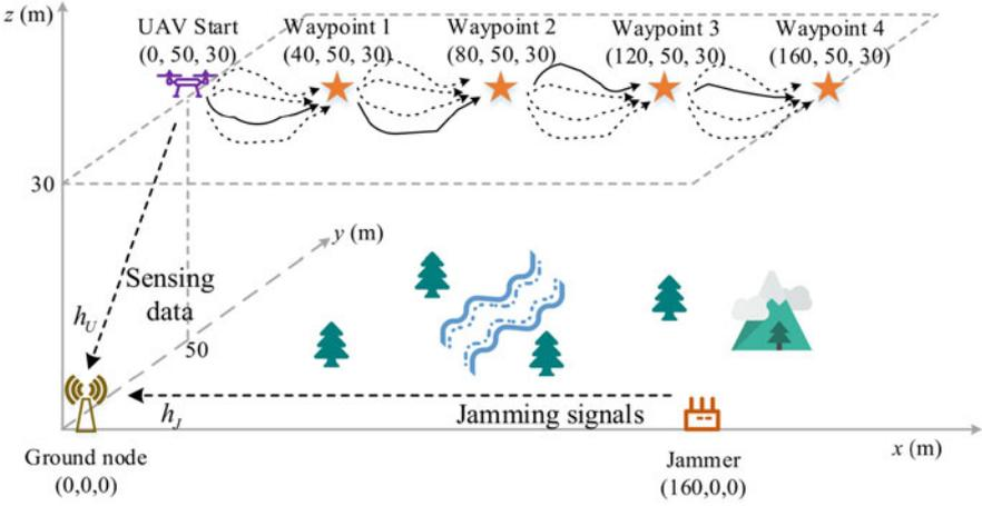
Fig. 2 Illustration of the simulation settings of the anti-jamming UAV communication network
