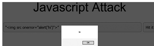
FIGURE 13.4 Our page when we input the command <img src onerror = "alert('hi')"> .
